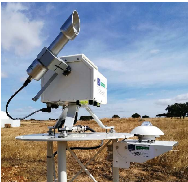
Fig. 7. General view of the direct and global radiation measuring equipment.
